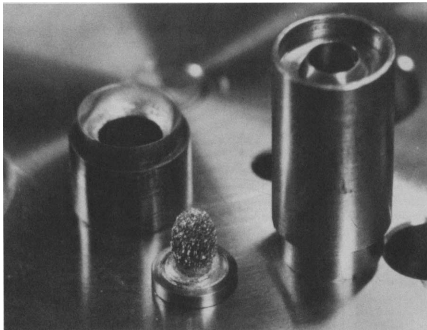
FIG. 12. Distilled Am metal (2 g) (center, front) and associated parts of the Ta still.
