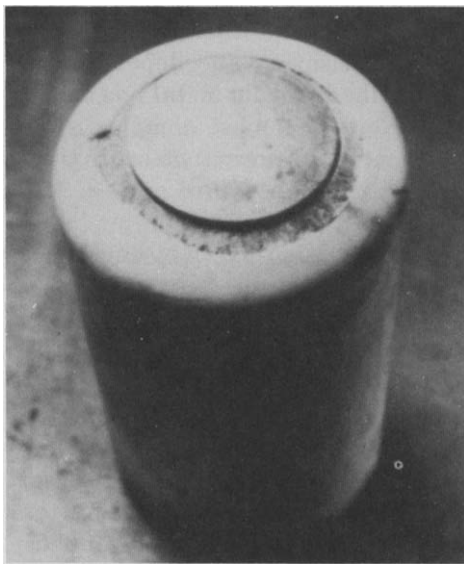
FIG. 9. Photograph of a typical Pu metal product from the DOR process.
